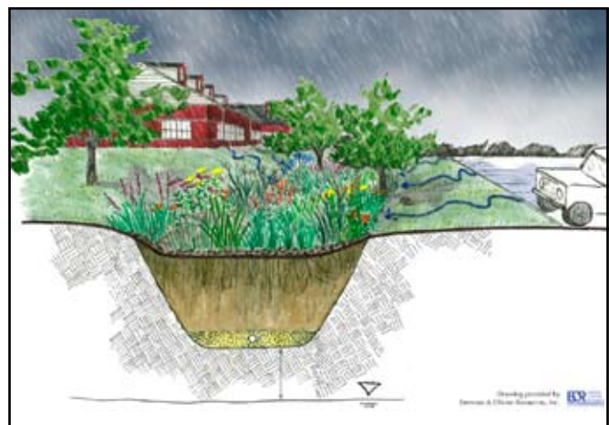
Following Storm Event - Remaining storage draw- down
